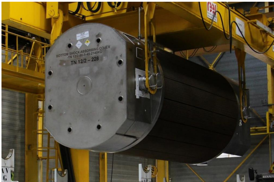
Figure 1. ORANO TN12/2 cask for the transport of spent fuel assemblies
