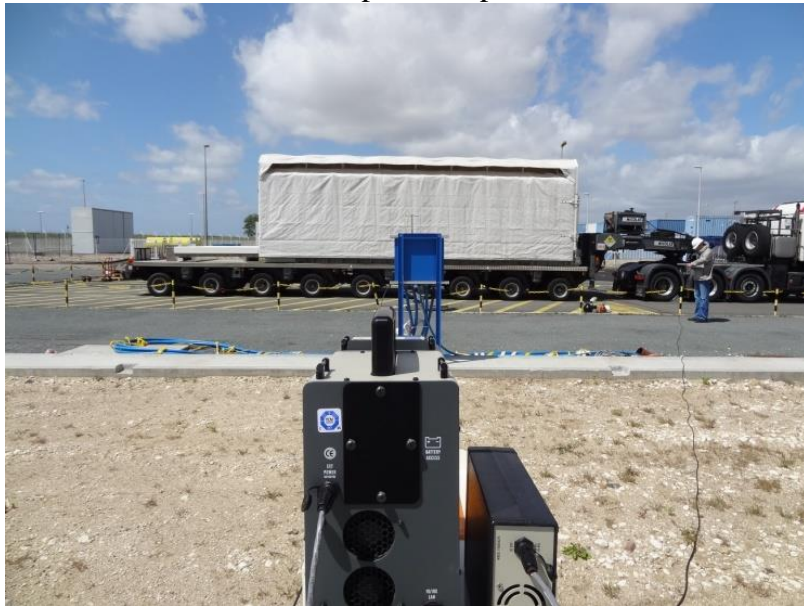
Figure 2. Spectrometry measures on an ORANO TN12/2 at BLAYAIS NPP
