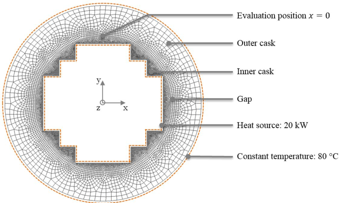
**Figure 2. Simplified verification model including boundary conditions and evaluation position**
