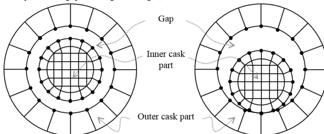
**Figure 1. Schematic cask in interim storage configuration (annular gap, left) and transport configuration (asymmetric gap, right)**
