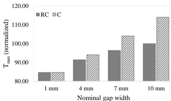
**Figure 3. Influence of the type of heat transfer (RC: radiation and conduction; C: conduction only) in the gap as a function of the gap width for a cask in transport configuration**
