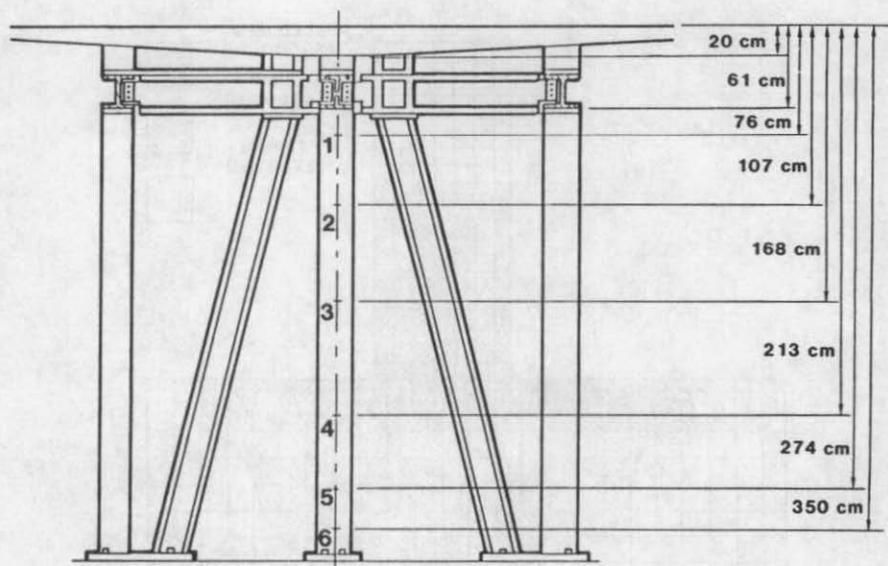
FIG. 4. Strain gauge locations on centre load spreading column.
