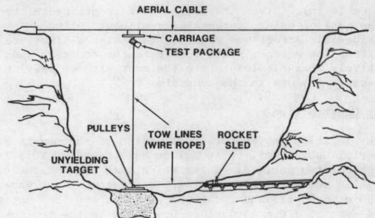
FIG. 2. Rocket Pulldown Facility.
