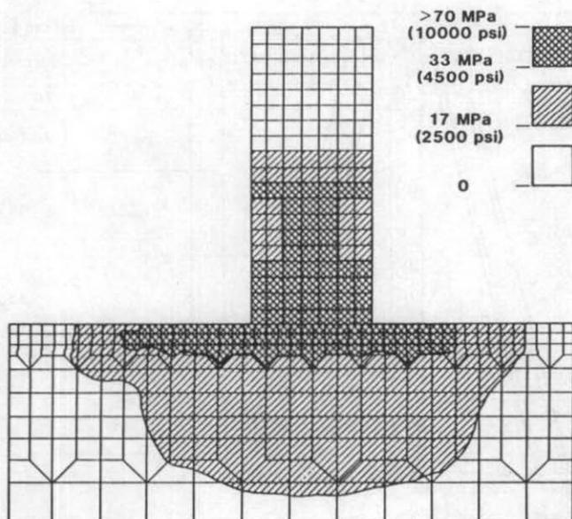
FIG. 3. Von Mises' stress in target and test unit calculated by DYNA2D finite element code.
