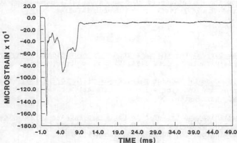
FIG. 5. Strain gauge signal at 76 cm below top of armour.
