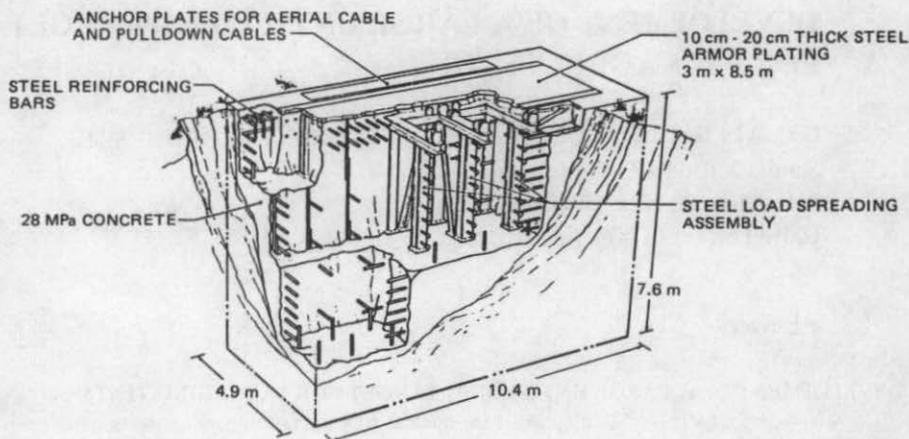
FIG. 1. 910 t armoured target at Sandia National Laboratories.
