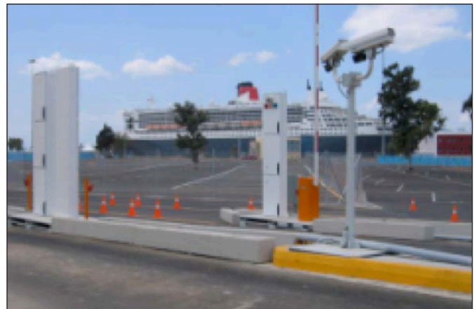
Figure 1. Radiation detection equipment at Piraeus Seaport (top) and at the extra-Schengen Passengers Terminal of the International Airport of Athens (bottom)
