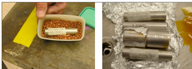
Figure 1. Certified Pu-238 sealed sources
