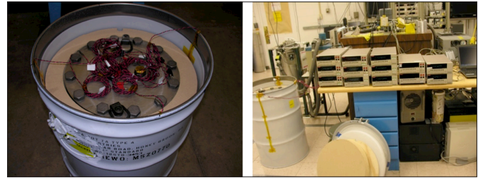
Figure 6. Testing setup, POC wired up (left) and volt meters along with MultiCal program (right)
