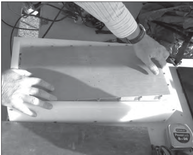
Figure 7. ^6\text{Li} -loaded glass fiber neutron detector and associated high-density polyethylene (HDPE) moderator enclosure
