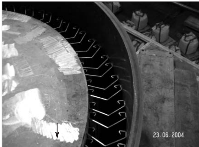
Figure 1. Copper heat conducting elements between the liners of the cask body
