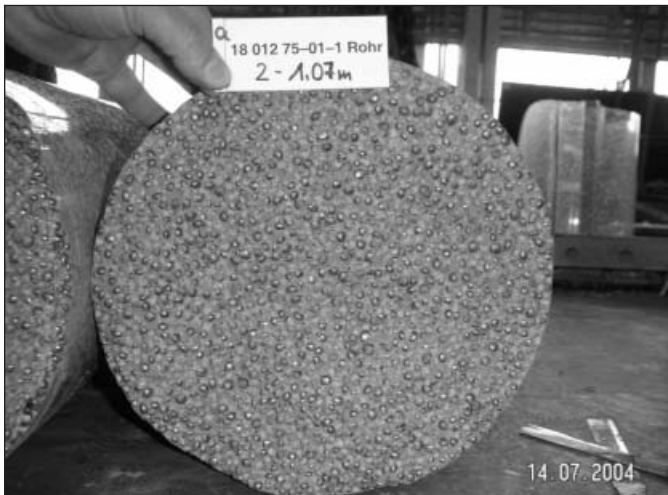
Figure 2. CONSTORIT specimen between the liners of the cask body
