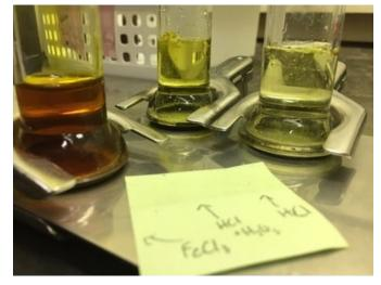
**Figure 3.** Setup used to complete the corrosion experiments. The hydrogen chloride (HCI) and ferric chloride (FeCI<sub>3</sub>) solutions are in the columns and were applied to one side of the 316L plates. (The mixture of hydrogen chloride [HCI] and hydrogen peroxide shown in the middle was not used because the response of the 316L to the solution was similar to that of HCI alone.)
