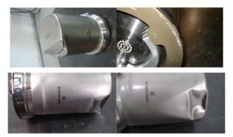
Figure 2. Examples of SAVY containers after drop testing was performed in compliance with regulations DOE M 441.1-1 and 49 CFR 173.465 requirements. External damage can be quantified; however, internal damage and cracking due to mechanical and corrosion processes cannot be determined using current destructive test methodologies.
