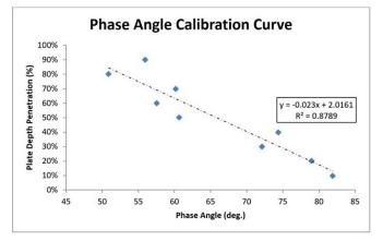
**Figure 10.** The measured phase angle plotted for each machined pit depth. The actual pit depths (percentage of plate thickness) are from the machined test plate.
