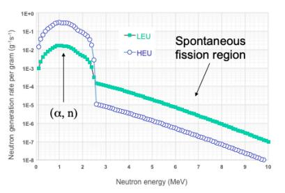
Figure 4. Neutron energy distribution displaying the alpha-n and spontaneous fission regions for both highly enriched uranium (HEU) and low enriched uranium (LEU)
