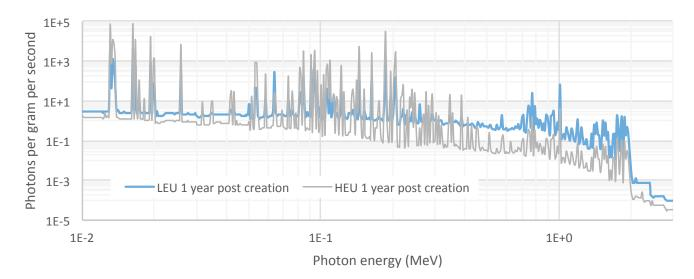
Figure 5. Gamma spectrum generated after 1 year of decay product ingrowth for LEU and HEU. This would be generated uniformly within the UF<sub>6</sub> material
