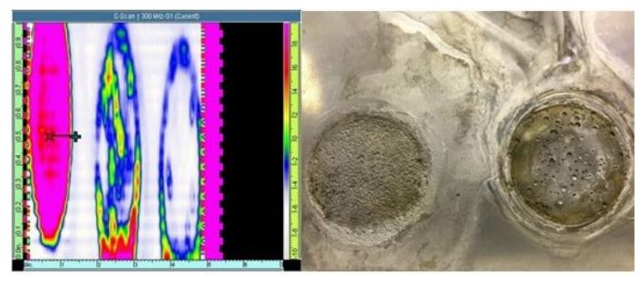
**Figure 9.** Example of ECA analysis of pitted 316L samples (right). The photograph on the right shows the 316L exposed to 3M and 1.5M FeCl<sub>3</sub>. The image on the left is a composite of three different samples: a baseline sample (uncorroded; seen as mostly pink), the sample exposed to 3M FeCl<sub>3</sub> in the middle, and the sample exposed to 1.5M FeCl<sub>3</sub>. The colors on the instrument can be adjusted to create a flaw (pitting) map.
