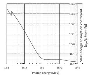
Figure 3. Mass energy absorption coefficient for a standard silica brick
