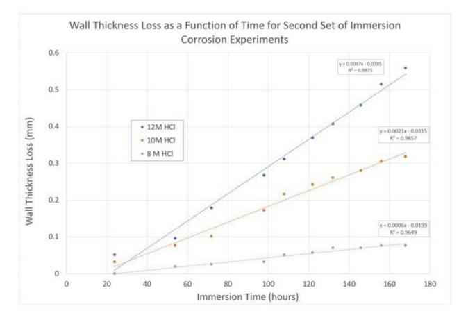
Figure 6. Wall thickness loss of thin 316L plates corroded with various concentrations of HCl over 7 days (168 hours). The points represent data collected by a UT gauge. However, the data from the UT gauge were within 2.5% of the values measured by a micrometer.
