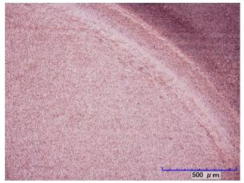
Figure 7. Digital microscope image of the edge of a circular region of a 316L plate treated with 12M HCl for 7 days.
