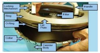
**Figure 1.** SAVY containers used for nuclear material storage at Los Alamos National Laboratory. (a) SAVY containers are available in various sizes, from 1 quart to 10 gallons. (b) The containers have various components, including a locking mechanism, HEPA filter, and a folding handle.
