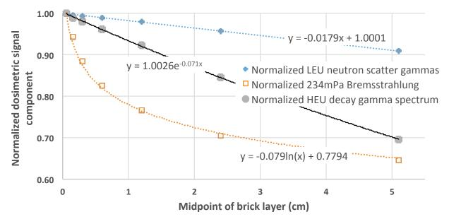
Figure 7. Attenuation description for dose in a material as a function of the material's thickness. The functional form and parameters of the fits are entirely arbitrary and only intended to demonstrate clear distinctions in attenuation profiles from different source terms
