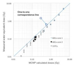
**Figure 2.** Measured doses shown as a function of expected doses based on Monte Carlo N-Particle Transport Code (MCNP) calculations. Values are obtained for different slices taken from separate cores, making three dose depth profiles<sup>1</sup>
