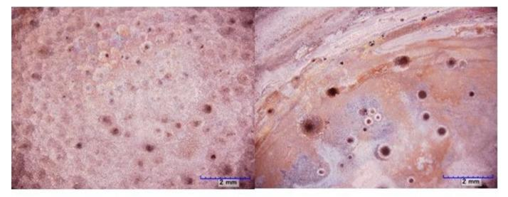
Figure 8. Samples corroded with FeCl<sub>3</sub> exhibiting pitting corrosion. The sample at left was treated with 3M FeCl<sub>3</sub>, and the sample at right was treated with 1.5M FeCl<sub>3</sub>.
