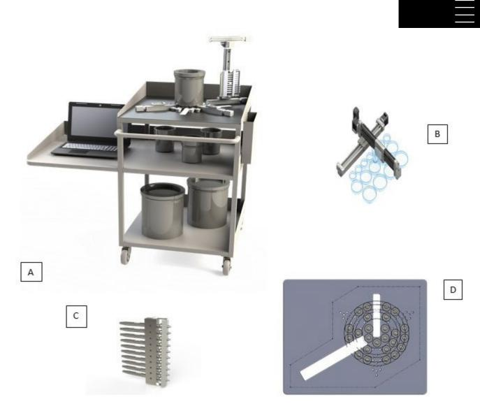
Figure 11. Proposed test setup for completing the nondestructive evaluations of the Hagan and SAVY containers. (a) Cart with the entire measurement setup, (b) raster base for the ECA, (c) multi-Sonopen assembly rack, and (d) plan view schematic of the adjustable baseplate to accommodate various container sizes.
