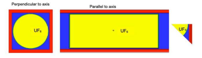
Figure 6. Equivalent geometry utilized to calculate dose deposition tallies in brick material originating from a 30B canister filled with UF<sub>6</sub>. The inset on the far right shows the actual sections with reflecting boundaries above and to the lower left with the canister also cut in half (and reflected) along its axis
