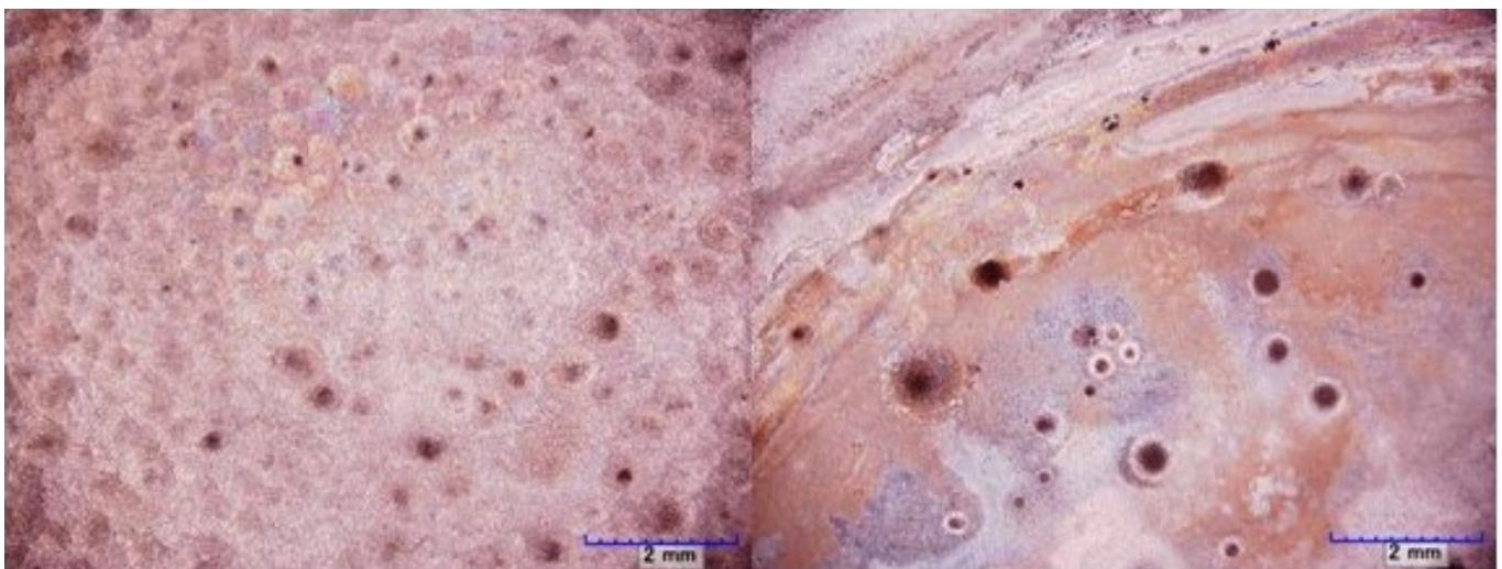
**Figure 8.** Samples corroded with  $\text{FeCl}_3$  exhibiting pitting corrosion. The sample at left was treated with 3M  $\text{FeCl}_3$ , and the sample at right was treated with 1.5M  $\text{FeCl}_3$ .
