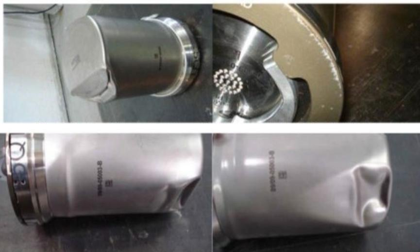
**Figure 2.** Examples of SAVY containers after drop testing was performed in compliance with regulations DOE M 441.1-1 and 49 CFR 173.465 requirements. External damage can be quantified; however, internal damage and cracking due to mechanical and corrosion processes cannot be determined using current destructive test methodologies.
