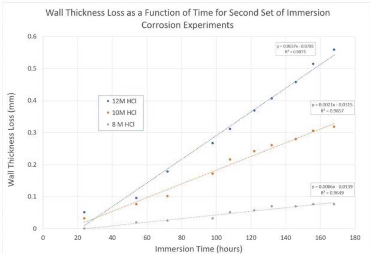
**Figure 6.** Wall thickness loss of thin 316L plates corroded with various concentrations of HCl over 7 days (168 hours). The points represent data collected by a UT gauge. However, the data from the UT gauge were within 2.5% of the values measured by a micrometer.
