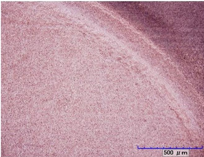
**Figure 7.** Digital microscope image of the edge of a circular region of a 316L plate treated with 12M HCl for 7 days.
