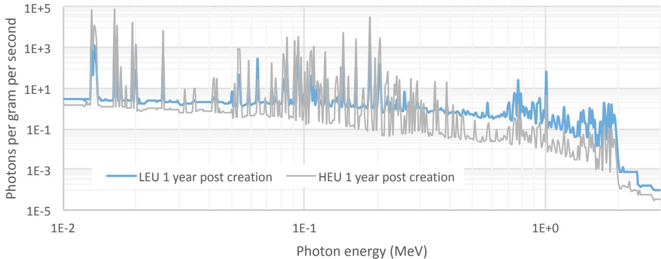
**Figure 5.** Gamma spectrum generated after 1 year of decay product ingrowth for LEU and HEU. This would be generated uniformly within the  $UF_6$  material
