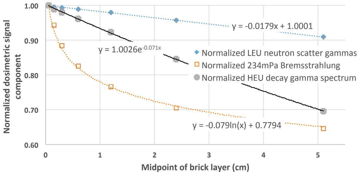
**Figure 7.** Attenuation description for dose in a material as a function of the material's thickness. The functional form and parameters of the fits are entirely arbitrary and only intended to demonstrate clear distinctions in attenuation profiles from different source terms
