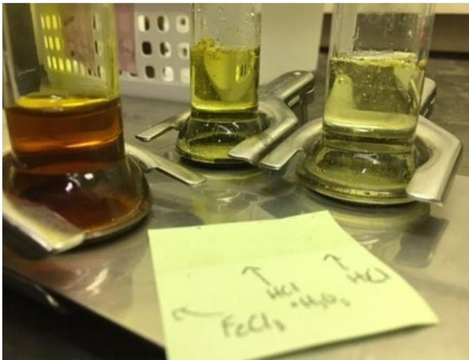
**Figure 3.** Setup used to complete the corrosion experiments. The hydrogen chloride (HCl) and ferric chloride ( $\text{FeCl}_3$ ) solutions are in the columns and were applied to one side of the 316L plates. (The mixture of hydrogen chloride [HCl] and hydrogen peroxide shown in the middle was not used because the response of the 316L to the solution was similar to that of HCl alone.)
