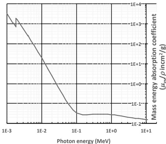
**Figure 3.** Mass energy absorption coefficient for a standard silica brick
