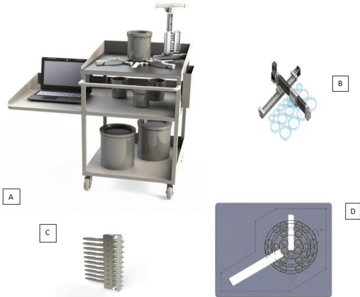
**Figure 11.** Proposed test setup for completing the nondestructive evaluations of the Hagan and SAVY containers. (a) Cart with the entire measurement setup, (b) raster base for the ECA, (c) multi-Sonopen assembly rack, and (d) plan view schematic of the adjustable baseplate to accommodate various container sizes.
