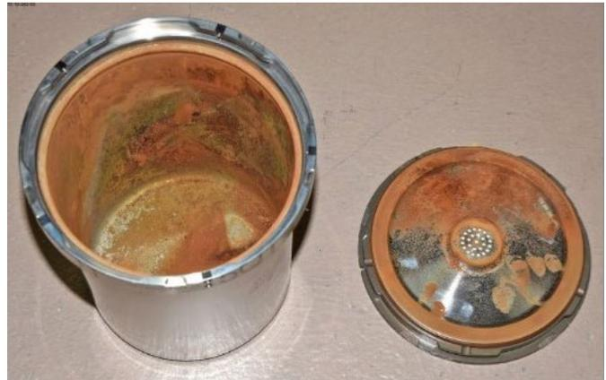
**Figure 4.** One of three corroded containers extracted from use as part of the surveillance program. This container had been in service for 13 months storing nuclear materials in an acidic environment. This container was inspected by the chosen NDT techniques.
