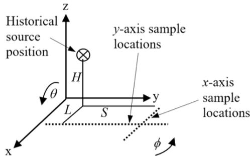
**Figure 1.** Coordinate definitions for dosimetric dependence on sample positions and depth for retrospective imaging and assay measurements
