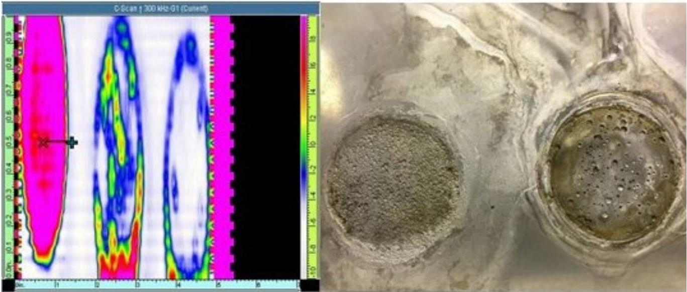
**Figure 9.** Example of ECA analysis of pitted 316L samples (right). The photograph on the right shows the 316L exposed to 3M and 1.5M  $\text{FeCl}_3$ . The image on the left is a composite of three different samples: a baseline sample (uncorroded; seen as mostly pink), the sample exposed to 3M  $\text{FeCl}_3$  in the middle, and the sample exposed to 1.5M  $\text{FeCl}_3$ . The colors on the instrument can be adjusted to create a flaw (pitting) map.
