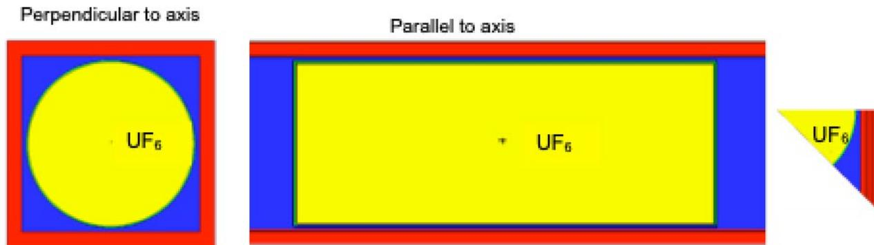
**Figure 6.** Equivalent geometry utilized to calculate dose deposition tallies in brick material originating from a 30B canister filled with  $UF_6$ . The inset on the far right shows the actual sections with reflecting boundaries above and to the lower left with the canister also cut in half (and reflected) along its axis
