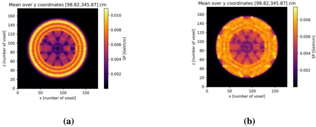
**Figure 10:  $\mu$ CT reconstruction of a simulation with three dummy bars: 2D-map of the SP mean in the central region of the DPC cask, obtained assuming a  $360^\circ$  detector coverage (a), and two  $60^\circ$ -acceptance modules, rotated around the cask in different positions (b).**
