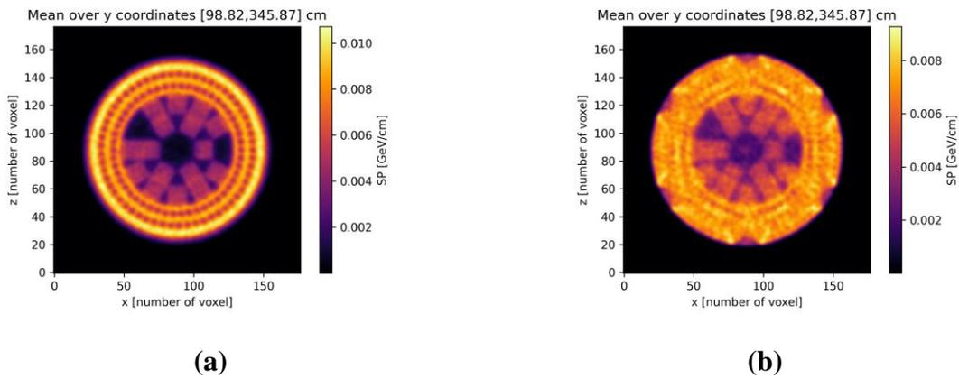
**Figure 9:  $\mu$ CT reconstruction of a simulation with three missing bars: 2D-map of the SP mean in the central region of the DPC cask, obtained assuming a  $360^\circ$  detector coverage (a), and two  $60^\circ$ -acceptance modules, rotated around the cask in different positions (b).**
