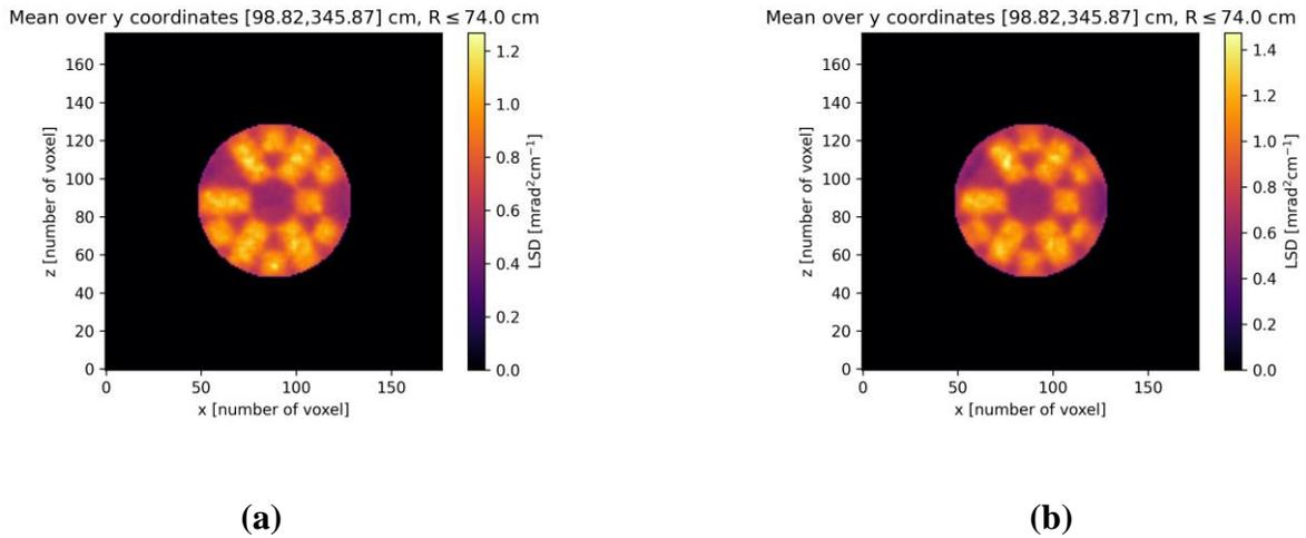
**Figure 11: MLEM reconstruction of a simulation with three missing bars: 2D-map of the LSD mean in the central region of the DPC cask, obtained assuming a 360° detector coverage (a), and two 60°-acceptance modules, rotated around the cask in different positions (b). The external shield is cut to avoid saturation.**
