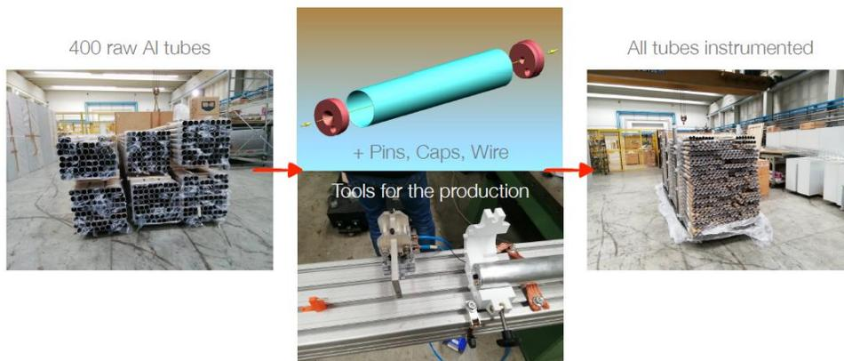
**Figure 4. Steps in tube production.**
