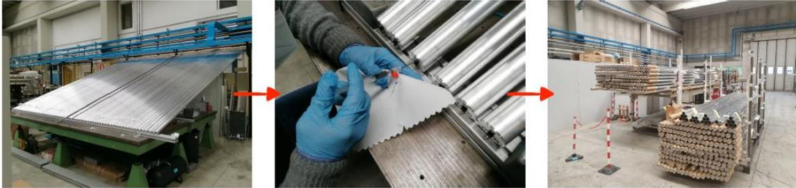
**Figure 5. Steps in cap gluing to complete tube readiness.**
