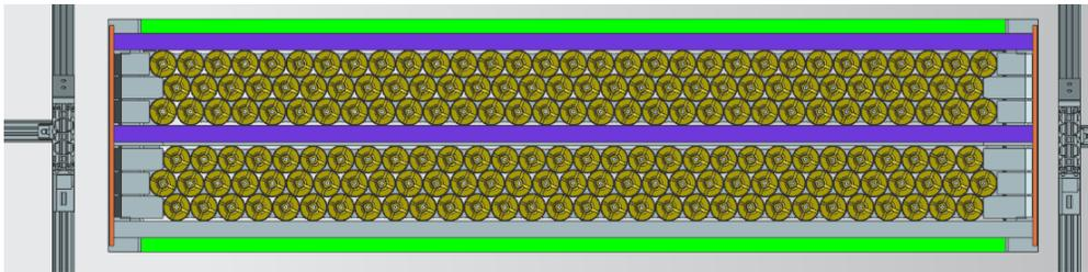
**Figure 2. Detailed view of a Muon Detector module assembled with six layers of drift tubes. The 3<sup>rd</sup> and 4<sup>th</sup> layers are separated in order to minimize the path ambiguities due to drift time circular symmetry.**
