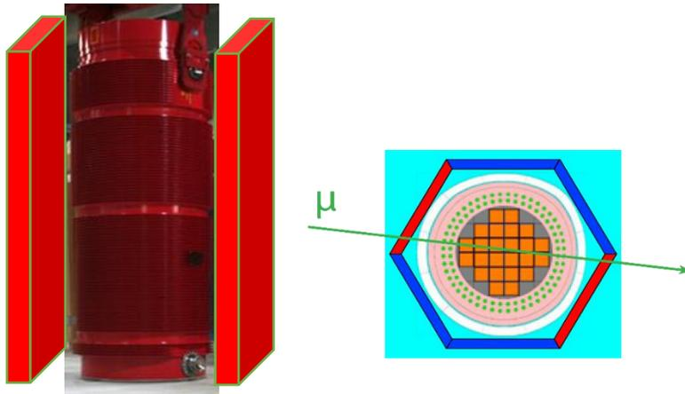
**Figure 1. Schematic view of a hexagonal 1/3 and full coverage Muon Detector (red and blue segments, respectively).**
