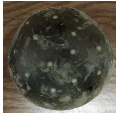
Figure 6. Surrogate fuel pebble with embedded microspheres
