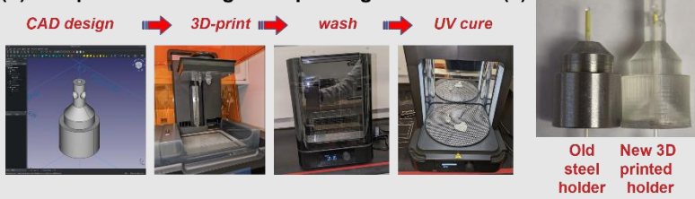
(b) Sample holder design and printing workflow (c)
