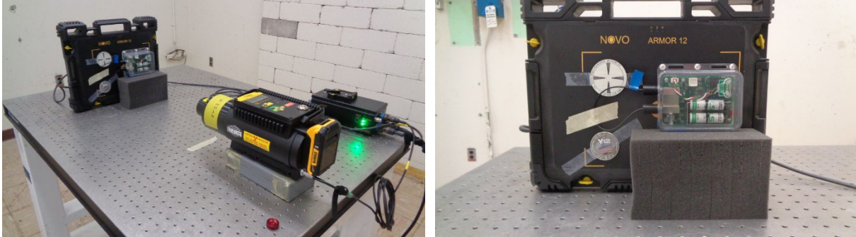
Figure 5. X-ray Radiography during Post-use Inspection Activities
