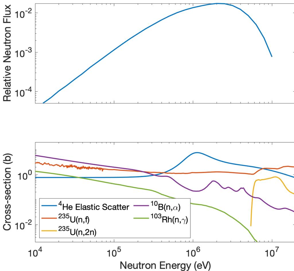
Figure 1: Typical fission neutron energy spectrum (above). Cross-sections of several reactions of interest for fast neutron detection (below). [3]
