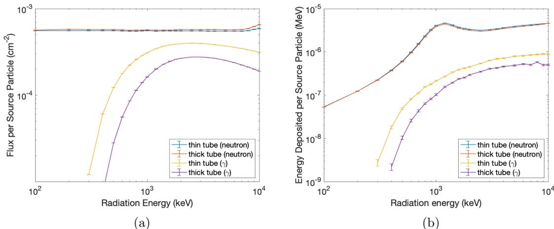
Figure 2: (a) Simulated neutron and gamma-ray flux inside each tube as a function of source radiation energy. (b) Simulated neutron and gamma-ray energy deposition in the active volume as a function of source radiation energy.
