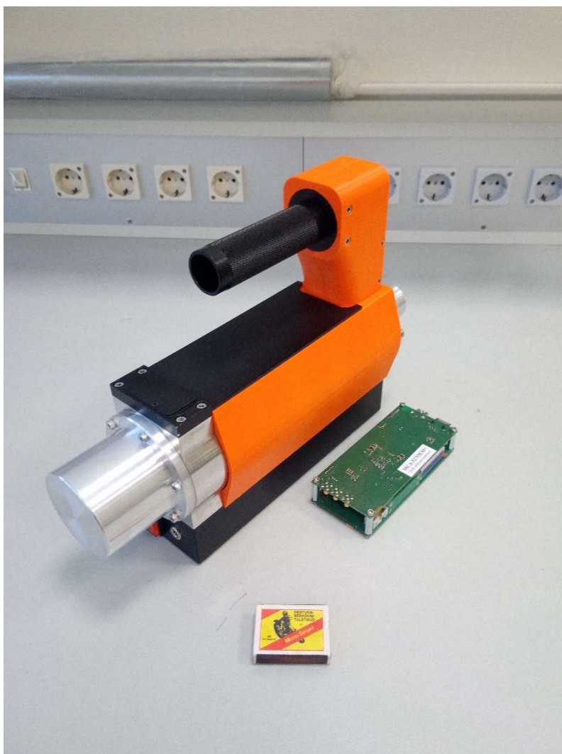
Figure 7 – RIGA with the MCA shown outside of the electronics housing for illustration.
