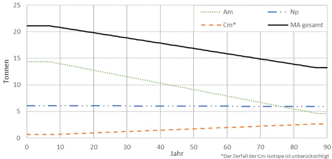
**Figure 2 shows the evolution of the different minor actinides in the scenario. Due the limitation imposed by the fixed fuel composition, only a small amount of minor actinides is actually fissioned in the scenario.**
