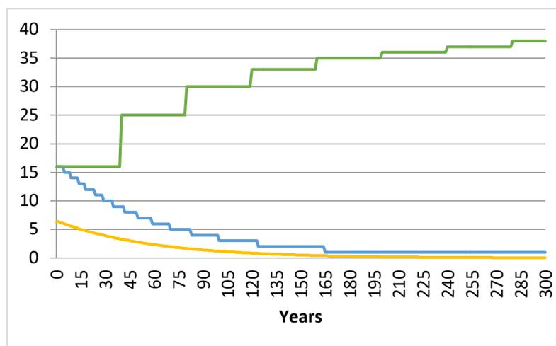
**Figure 1: Simple Scenario. Development of thermal power (yellow), required number of reactors (blue) and required total amount of reactors (green) for transmutation of 140 t TRU. The scenario is optimized for throughput as some reactors only operate for a few years.**
