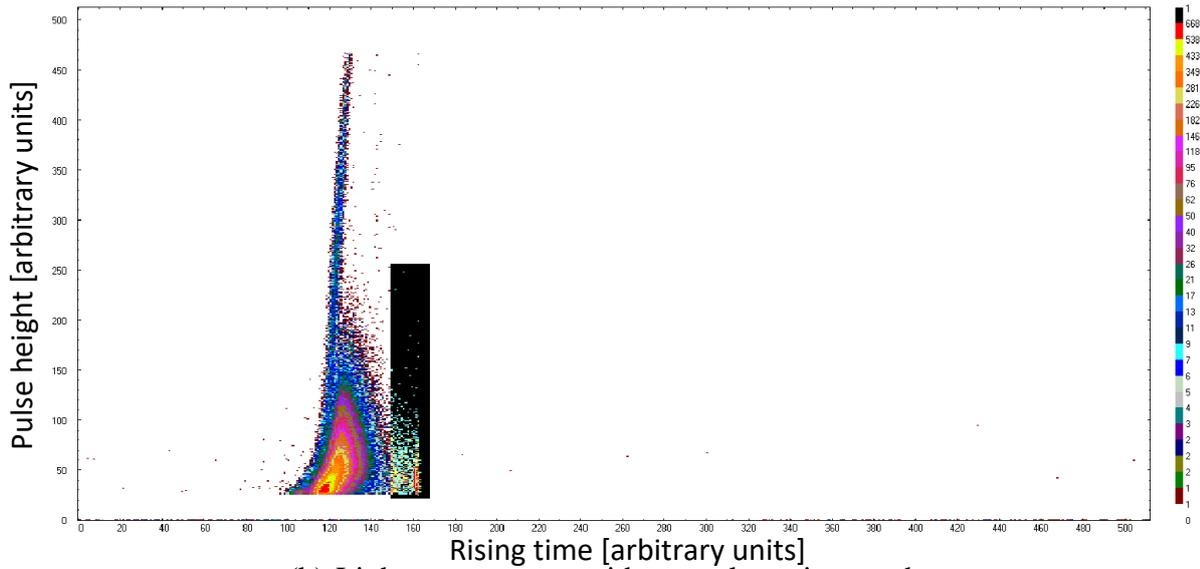
(b) Light output count with natural uranium as the target
