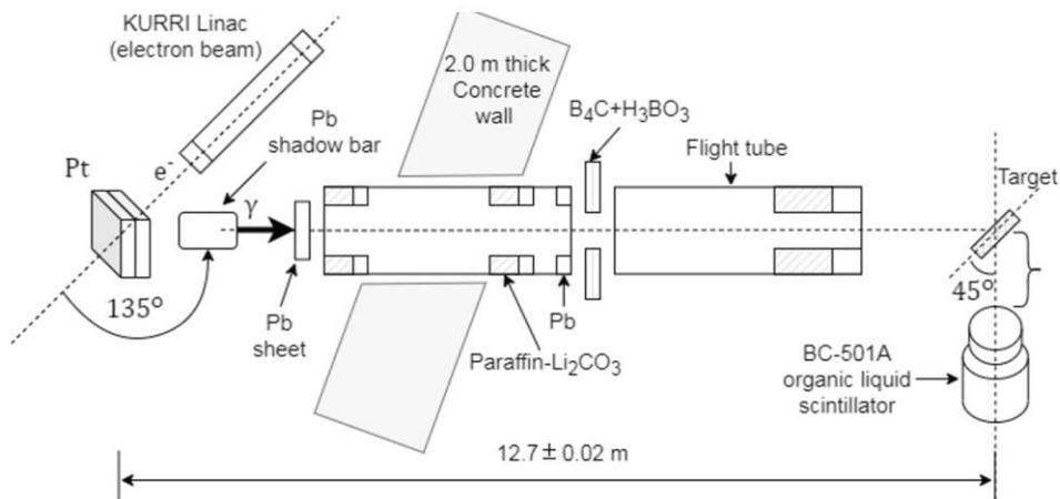
Figure 2: Experimental setup of KURRI Linac with BC-501A detector.
