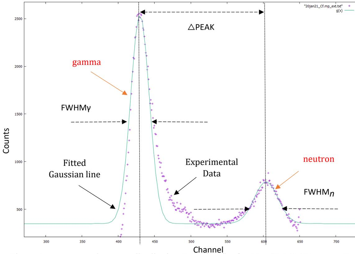
Figure 6: Neutron and gamma distribution Gaussian fits for 5'' x 5'' BC-501A scintillator.
