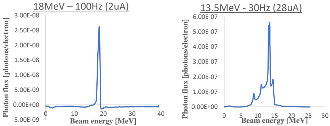
Figure 3: Beam profile of 18.0 and 13.5 MeV with different beam current.
