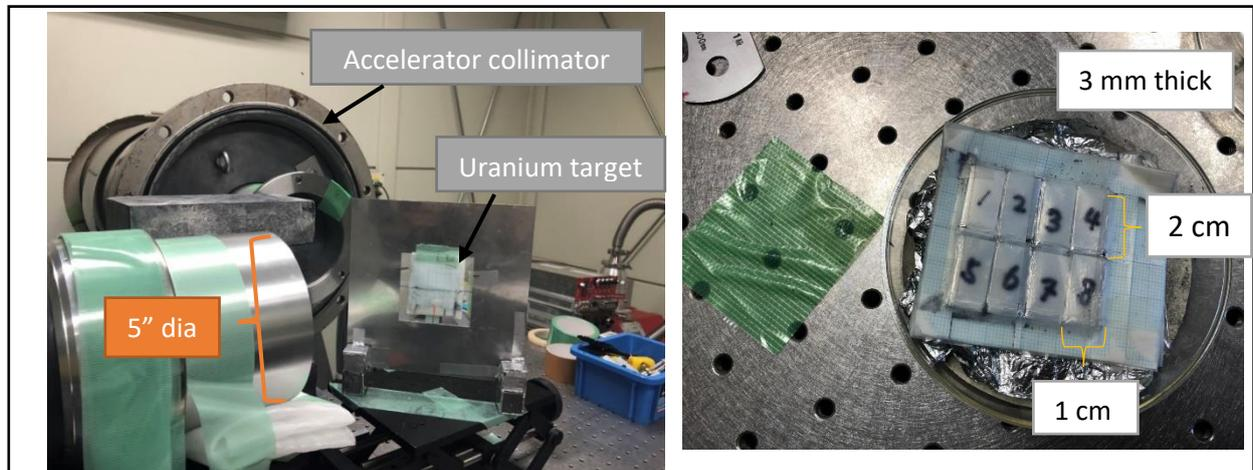
Figure 4 5'' x 5'' BC-501A and natural uranium target.
