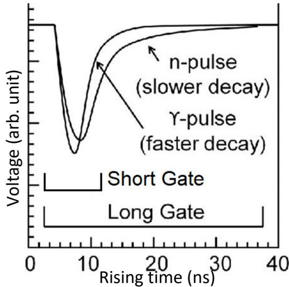
Figure 5: Depiction of the charge pulse difference for a neutron compared to a gamma.
