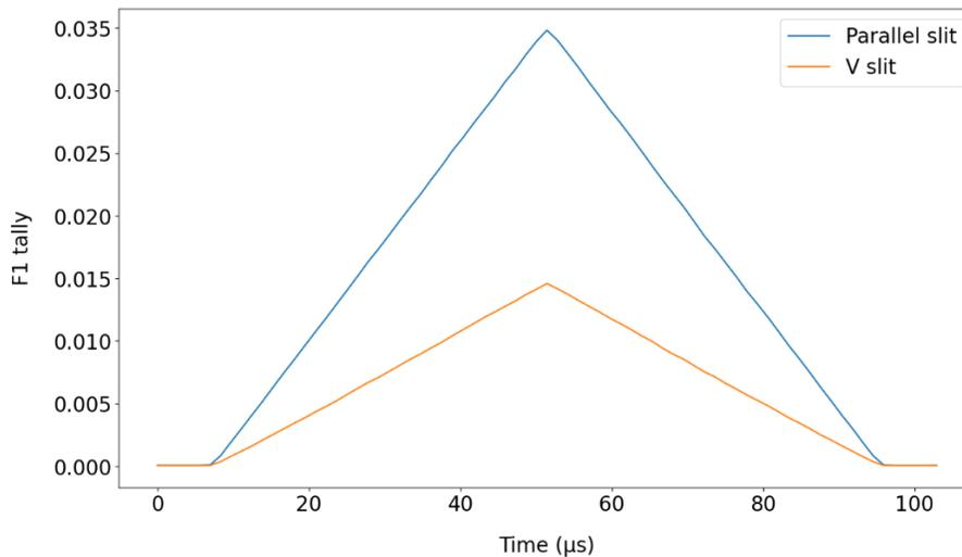
**Figure 3. MCNP simulated time-structured pulse for the source diameter = 4 cm.**
