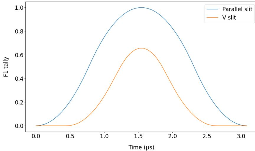
**Figure 2. MCNP simulated time-structured pulse for the source diameter = 0.07 cm.**
