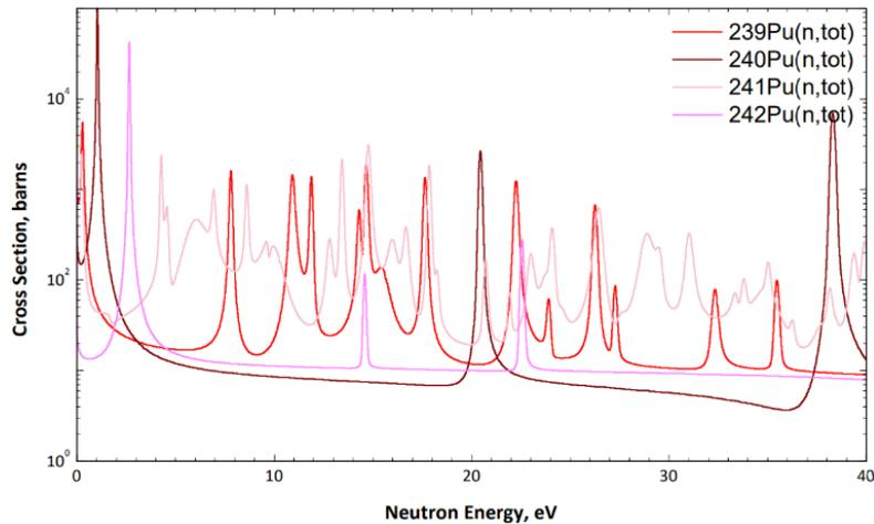
**Figure 1. ENDF/B-VII.1 total neutron cross-sections for isotopes of plutonium between 0.1 and 40 eV [3].**
