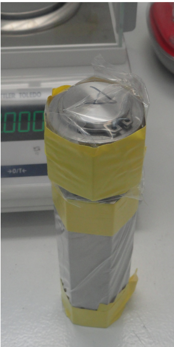
Figure 3. Plastic-protected bored-plug container. Protected container with funnel installed in preparation for filling with calcined ^{233}\text{U} oxide ( upper right ), with lid in place after removing plastic protecting threads ( left ), and during tightening using customized wrenches ( lower right ).
