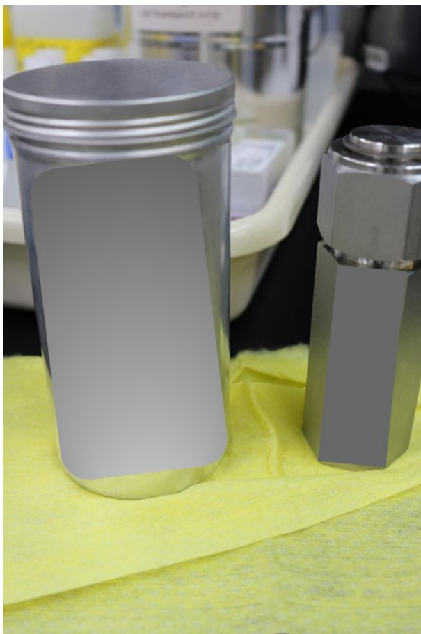
Figure 2. Typical specimen package. A Swagelok bored-plug container ( right ) serves as the primary specimen confinement and is overpacked in an aluminum screw-top container ( left ) with SS wool padding.
