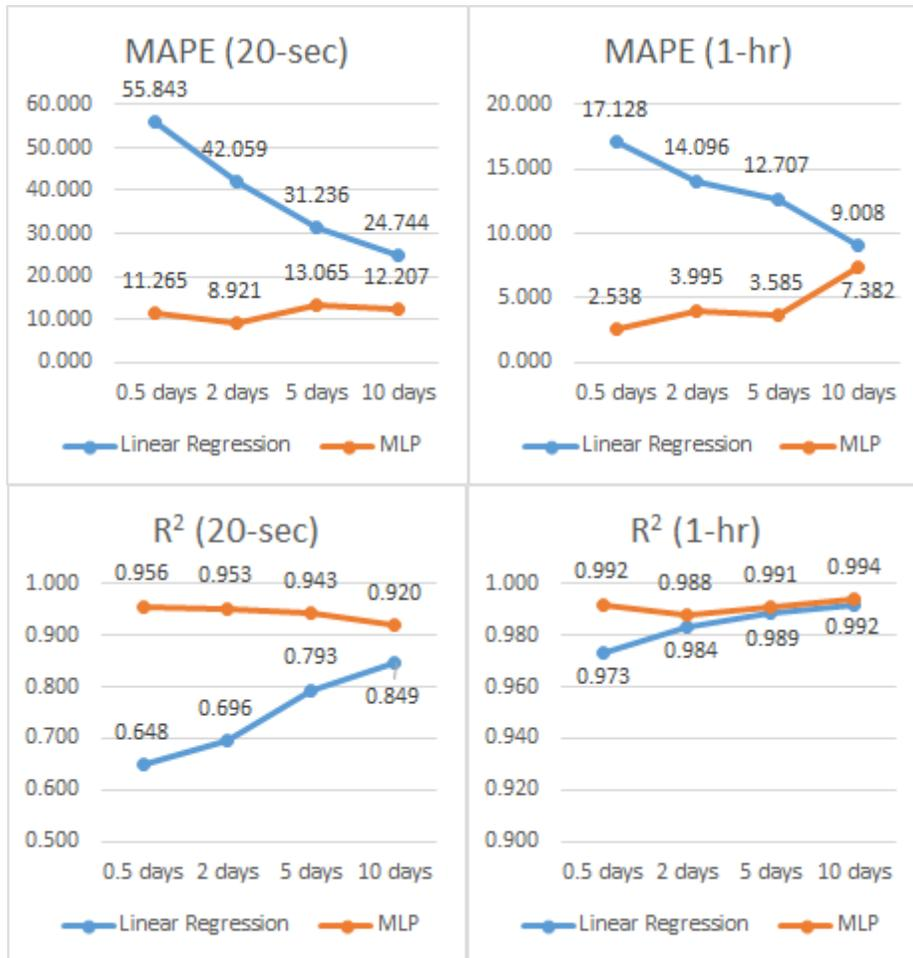
Figure 4. Predictive performance of standard linear regression and trained MLP model over different fuel cooling time and detector acquisition times.
