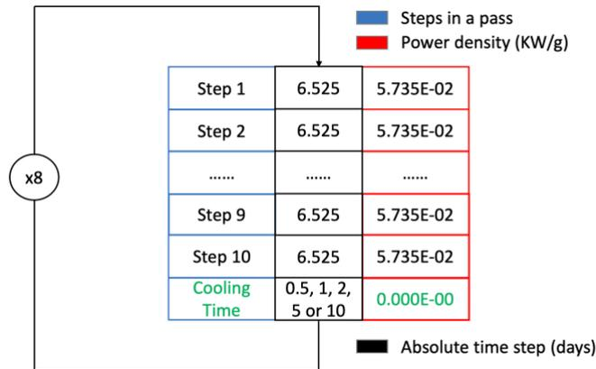
Figure 2. Illustration of the pebble lattice burnup process
