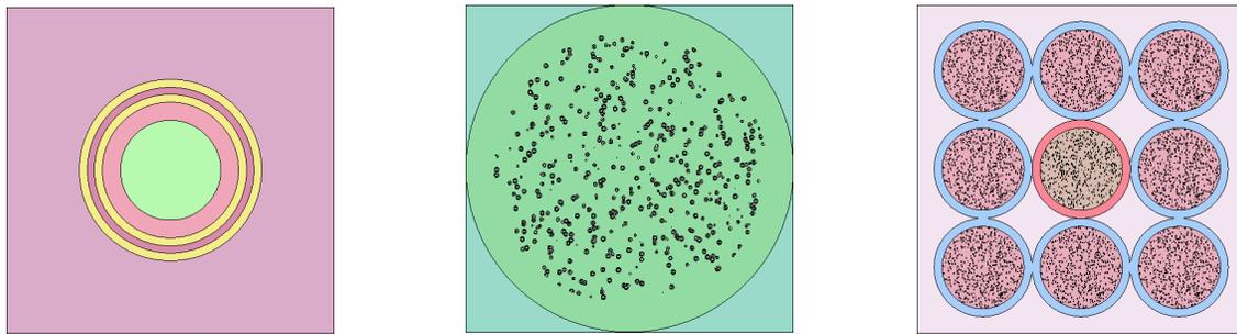
Figure 1. Model of a PBR fuel pebble from a TRISO (Left) to a pebble (Center) and a 3x3x3 Lattice (Right)
