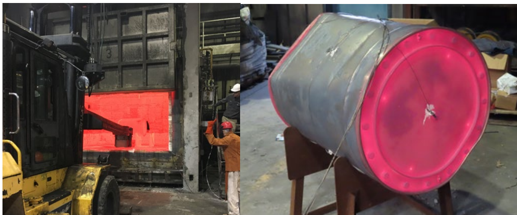
Figure 7. Test unit furnace removal and cooling
