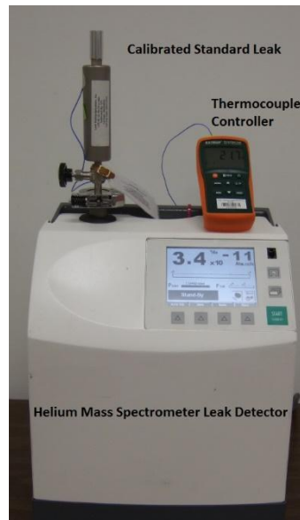
Figure 2. An Instrument Calibration, Standardization, or Verification of Calibration. (Note, the calibrated standard leak may be external, as illustrated here, or internal to the instrument.)
