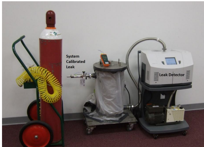
Figure 3. A Test System Calibration including a System Calibrated Leak Standard, Test Instrument, Test Object, and the Interconnecting Hardware.
