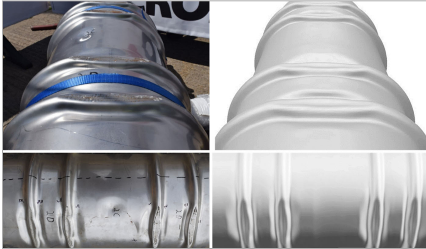
Figure 8. 9m side drop – deformation in the test (left) vs deformation in the analysis (right)
