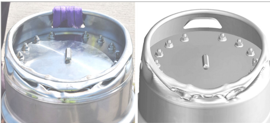
Figure 6. 9m lid edge drop – deformation in the test (left) vs deformation in the analysis (right)
