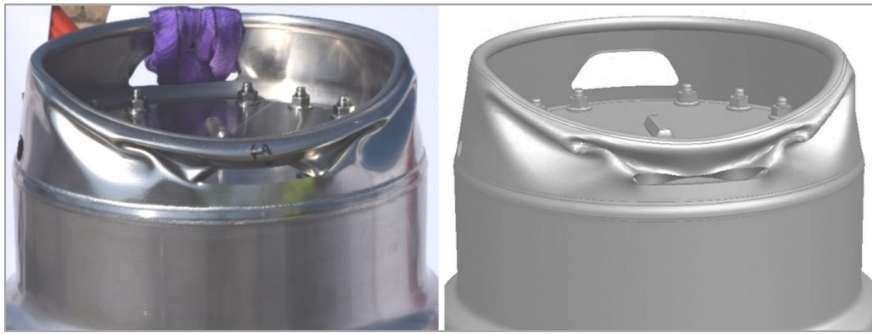
Figure 5. 1.2m lid edge drop – deformation in the test (left) vs deformation in the analysis (right)
