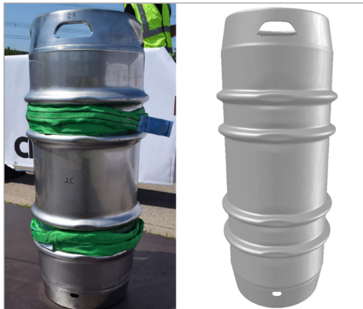
Figure 7. 1.2m side drop – deformation in the test (left) vs deformation in the analysis (right)
