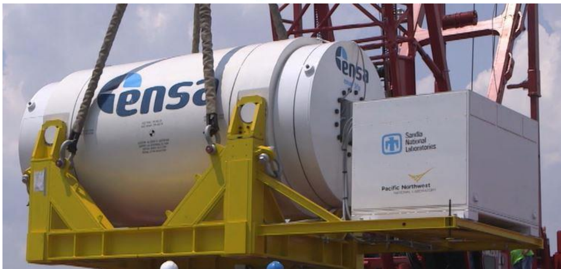
Figure 4. Test configuration for the Multi-Modal Surrogate Spent Nuclear Fuel Transportation Test
