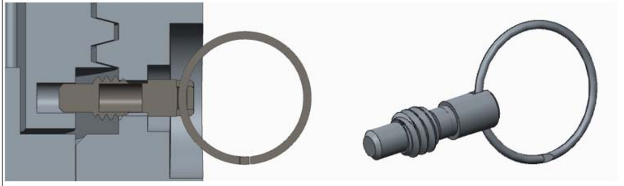
Figure 4. Containment Vessel Assembly Alignment Method
