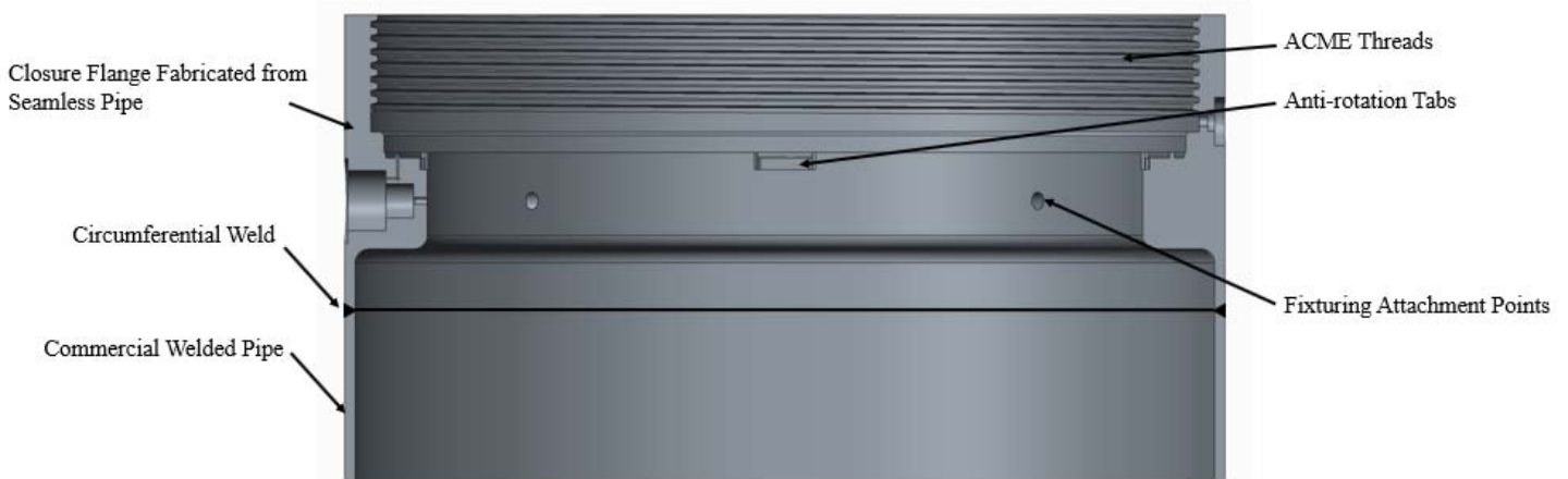
Figure 2. Containment Vessel Flange
