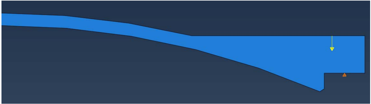
Figure 7. Package Lid Loading Conditions
