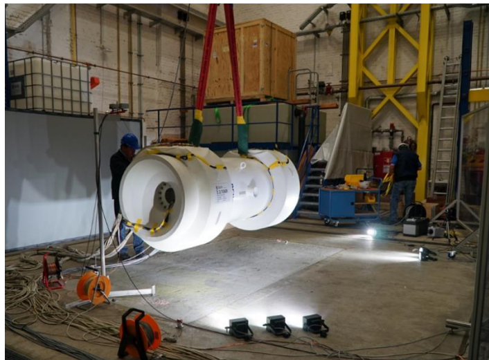
Figure 10. 30 cm drop test set up before the first drop (December 11, 2018).
