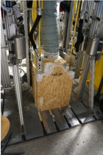
Figure 11. LLD - Setup during the tempering phase (outdoor unit)
