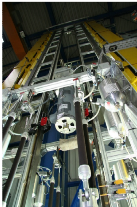
Figure 1. Assembly parts of BAM's Test Bench for Guided Drop Tests
