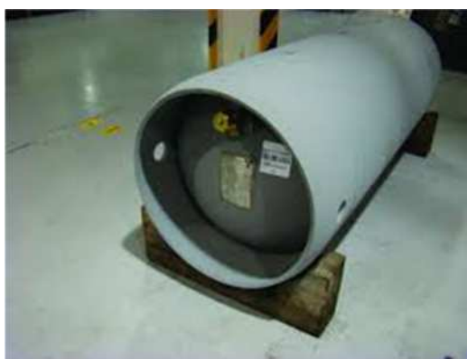
Figure 1 - A cylinder 30B (external diameter: 762 mm, total length: 2070 mm, internal volume: 736 litres)
