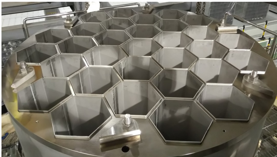
Figure 7 First Unit Fabrication of the 31VTH Basket, 95% Complete
