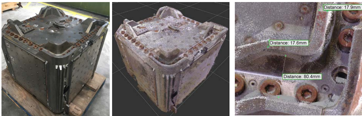
Figure 5 – 1/3 Scale Model (Left), Point Cloud Model (Middle), Verification Measurements (Right)
