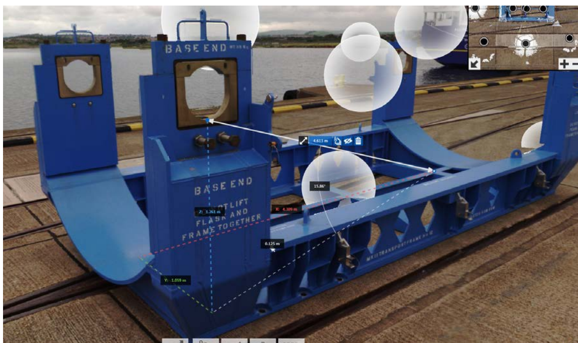
Figure 4 - Point cloud of Transport Frame overlaid with photography
