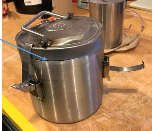
Figure 8. Latch container post drop deformation
