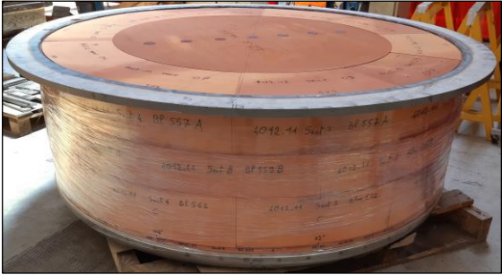
Figure 8: R83's impact limiter manufacturing (FENSOL™ foams)
