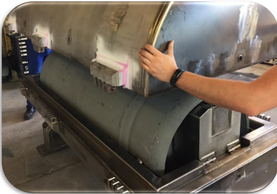
Figure 10. Closing of the DN30 after it had been loaded with a dummy cylinder
