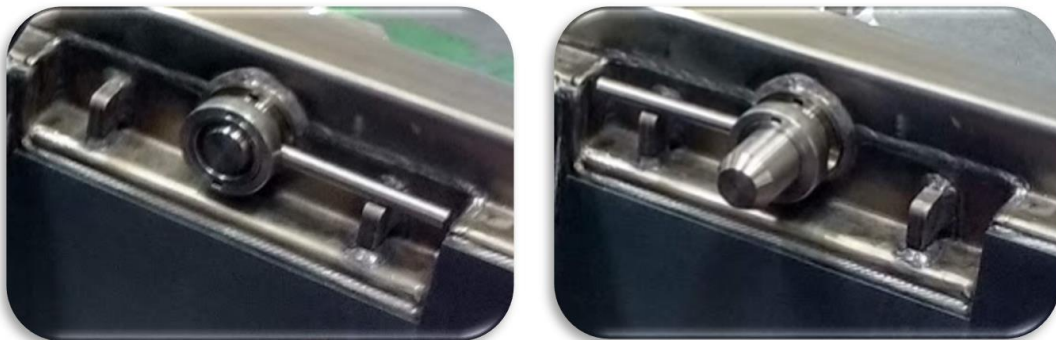
Figure 6. Operation of the DN30 anti-rotation devices (left: open position, right: locking position)
