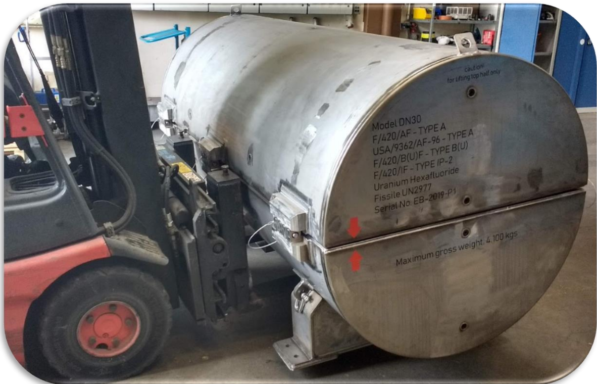
Figure 11. Lifting of the DN30 by means of a forklift
