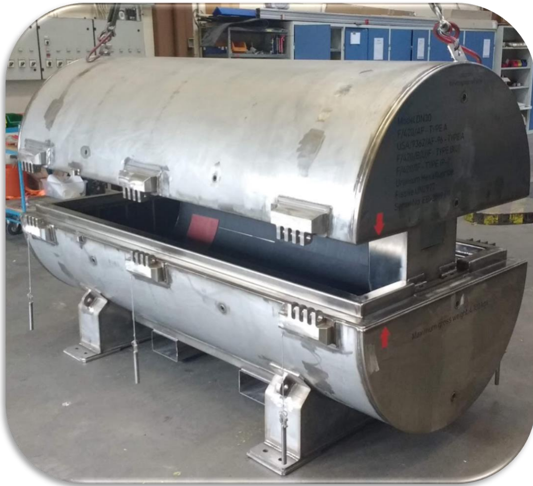
Figure 8. Lowering of the DN30 top half onto the DN30 bottom half
