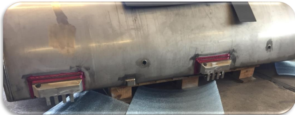
Figure 4. Dye penetrant test of the welds of the closure devices of the DN30 top half
