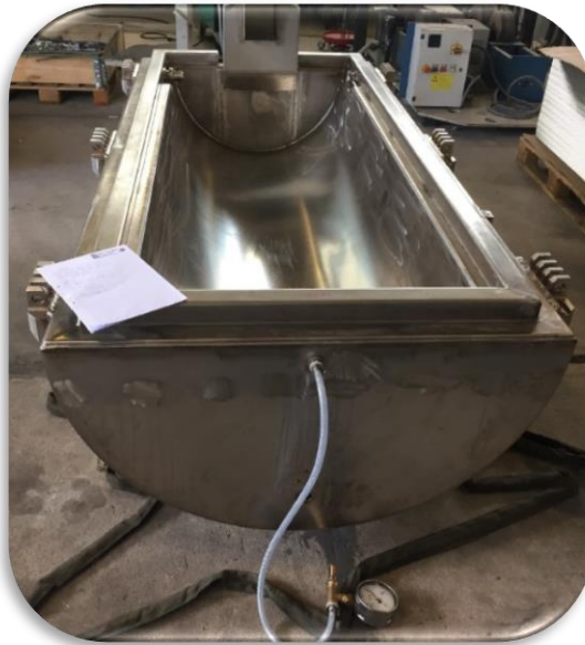
Figure 3. Leak test of the DN30 bottom half
