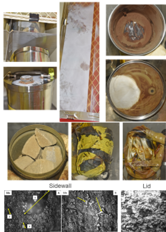
Figure 4. Photographs and photomicrographs of corrosion in a Hagan container (304L SS) resulting from a high americium salt residue packaged in a PVC bag.
