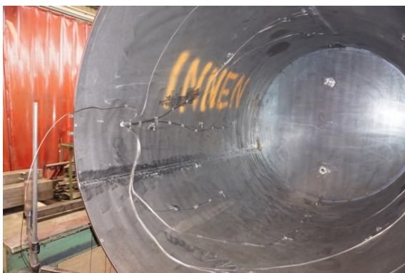
FIGURE 2. Thermocouples at the surface of the inner wall and detail of a thermocouple installation.
