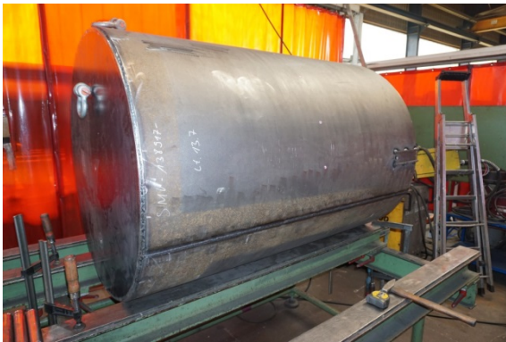
FIGURE 1. Manufacturing of the cylindrical reference package and filling of the cavity with insulation material after instrumentation with thermocouples.
