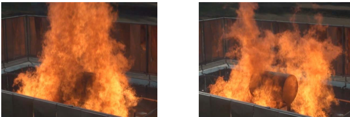
FIGURE 5. Typical flame engulfment situations during test no 18011.
