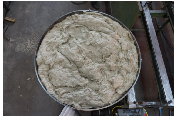
FIGURE 1. Manufacturing of the cylindrical reference package and filling of the cavity with insulation material after instrumentation with thermocouples.
