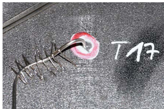
FIGURE 2. Thermocouples at the surface of the inner wall and detail of a thermocouple installation.
