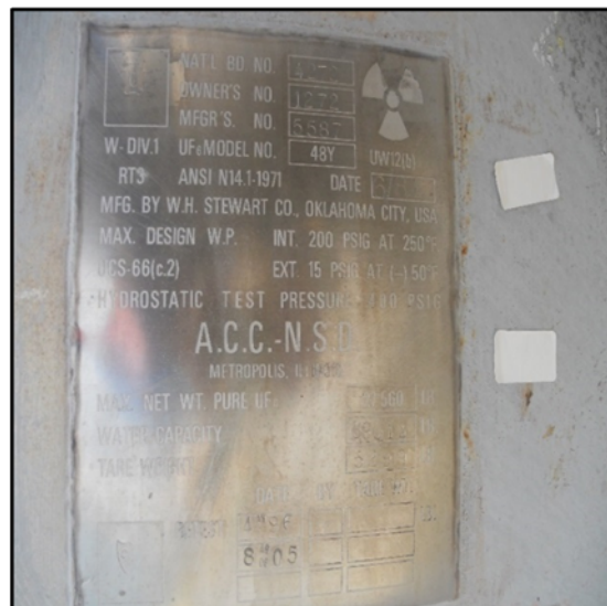
Figure 2. Representative nameplate welded to the end of a cylinder.
