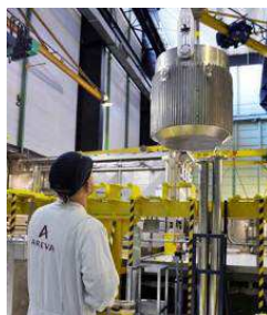
Fig.10: Cask handling to the preparation cell, before unloading
