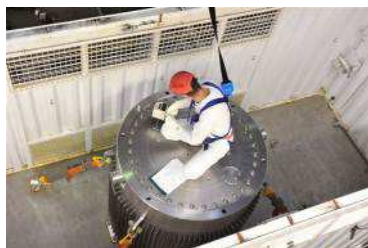
Fig.9: Radiological control on RRSF from transportation cask, without shock absorber pool
