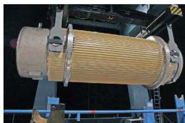
Fig.32: AREVA TN-81 dual purpose cask
