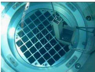
Fig.2: TN-MTR wet loading at RR site
