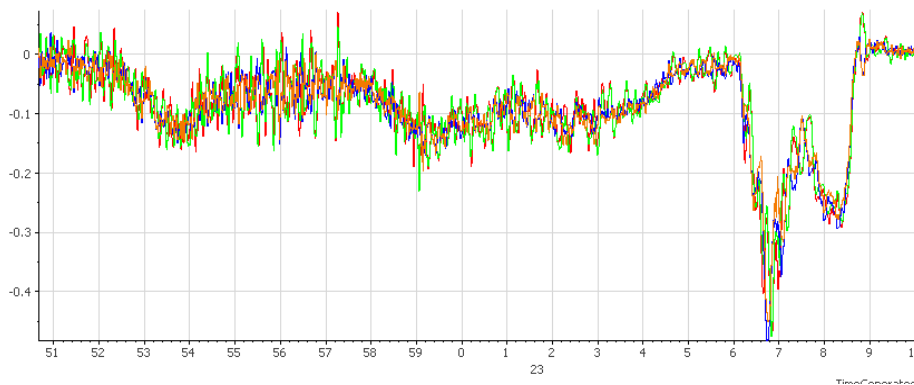
Figure 19: Longitudinal accelerations during sudden breaking (acceleration in g, time in s, x axis, superimposition of the 4 sensors)
