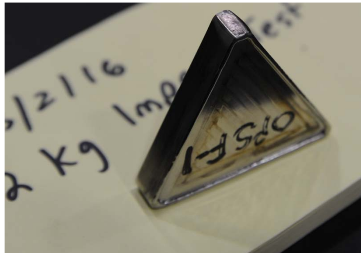
Figure 5 ZipCan vertex impact test result.
