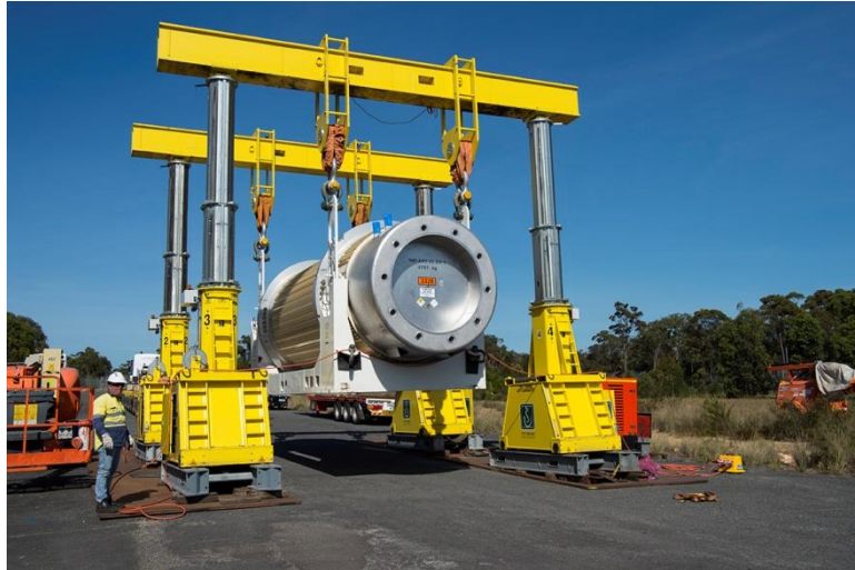
Figure 3 Gantry crane lift of TN81
