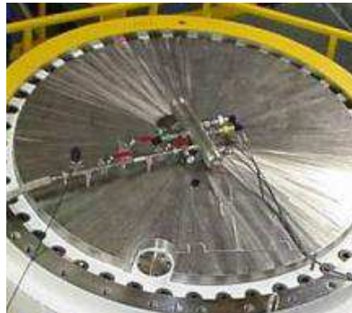
Figure5: Preparation of monitoring system on TN ® 24 casks
