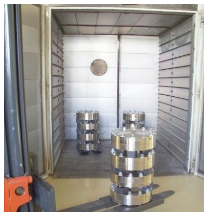
Figure 3: Test principle: Left side – mockup under the press. Right side – mockups piled up inside a furnace
