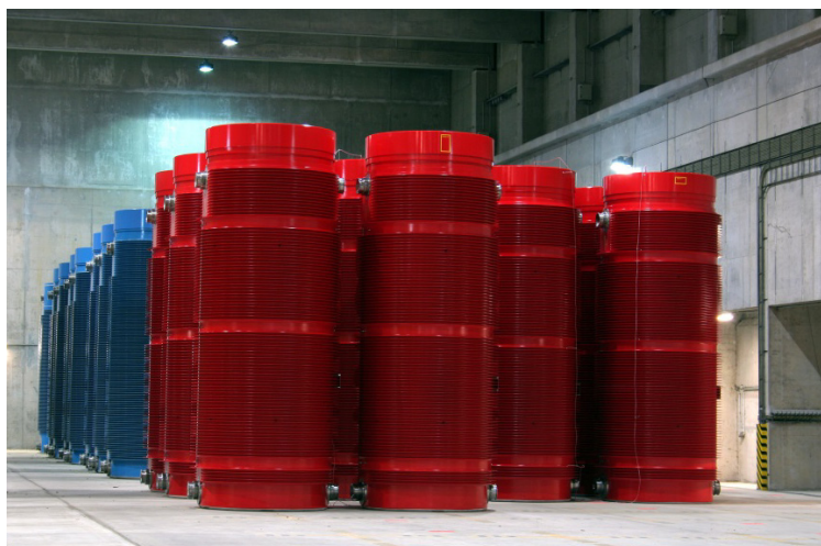
Figure 1 DPC CASTOR® HAW28M at Gorleben storage facility
