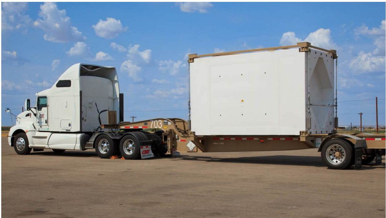
Figure 3. TRUPACT-III in Transport Mode
