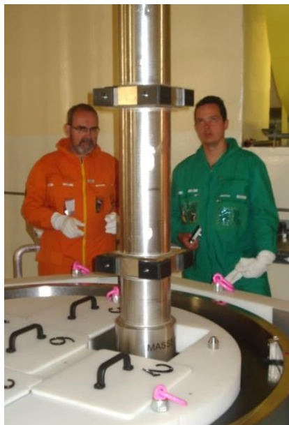
Photo 6: removing MOX assembly through the protective cover
