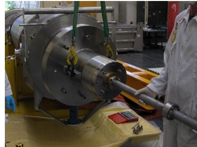
Figure 4 – Guillotine system and clock for plug removal
