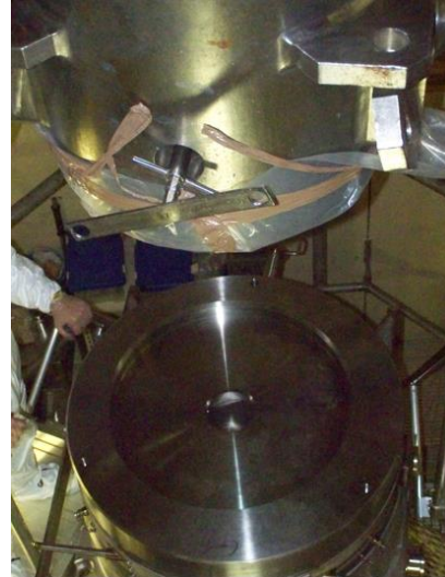
Figure 6 – Docking of lead castle onto transport packaging
