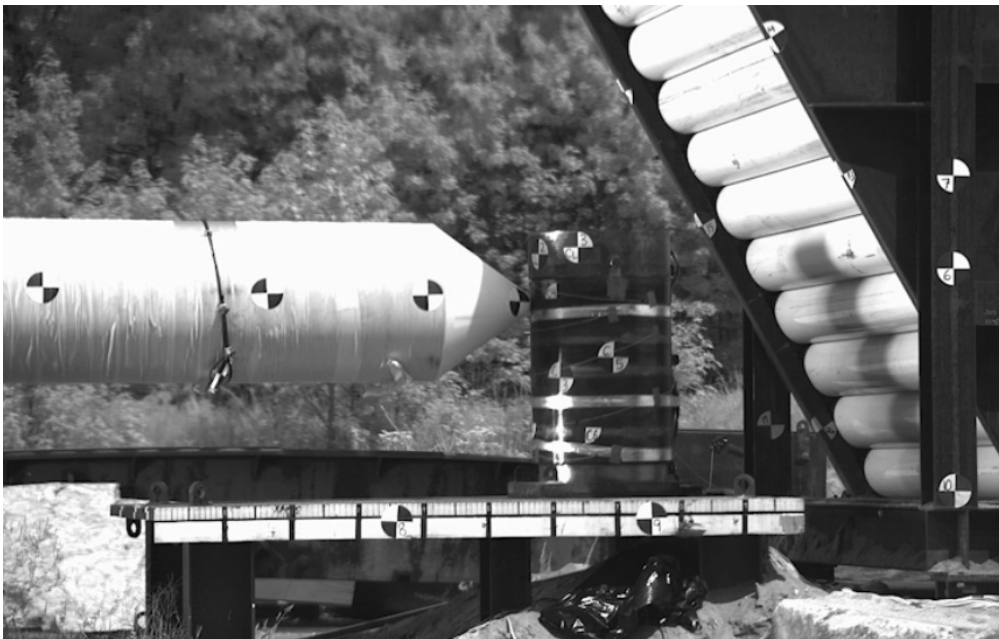
Figure 3 Missile just before Impact on Cask
