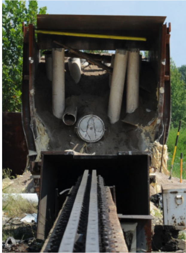
Figure 4 Cask in the catch box after Impact: Good Alignment of the Final Location of the Impacted Cask with the Rail Due to a Symmetric Impact by the Missile
