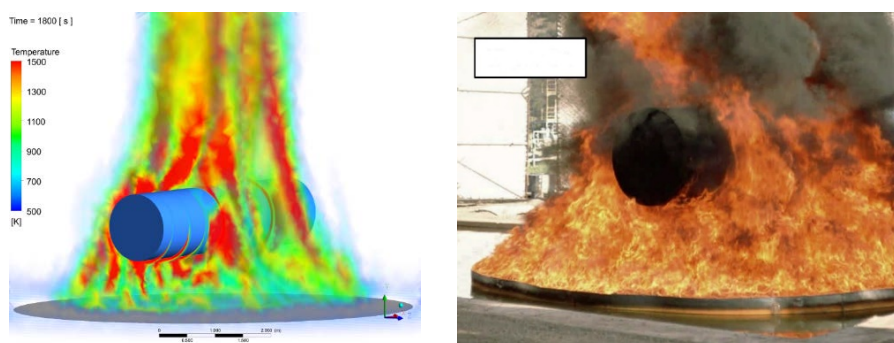
Figure 1: Comparison of simulated pool fire (left) with experimental pool fire (right) [5]
