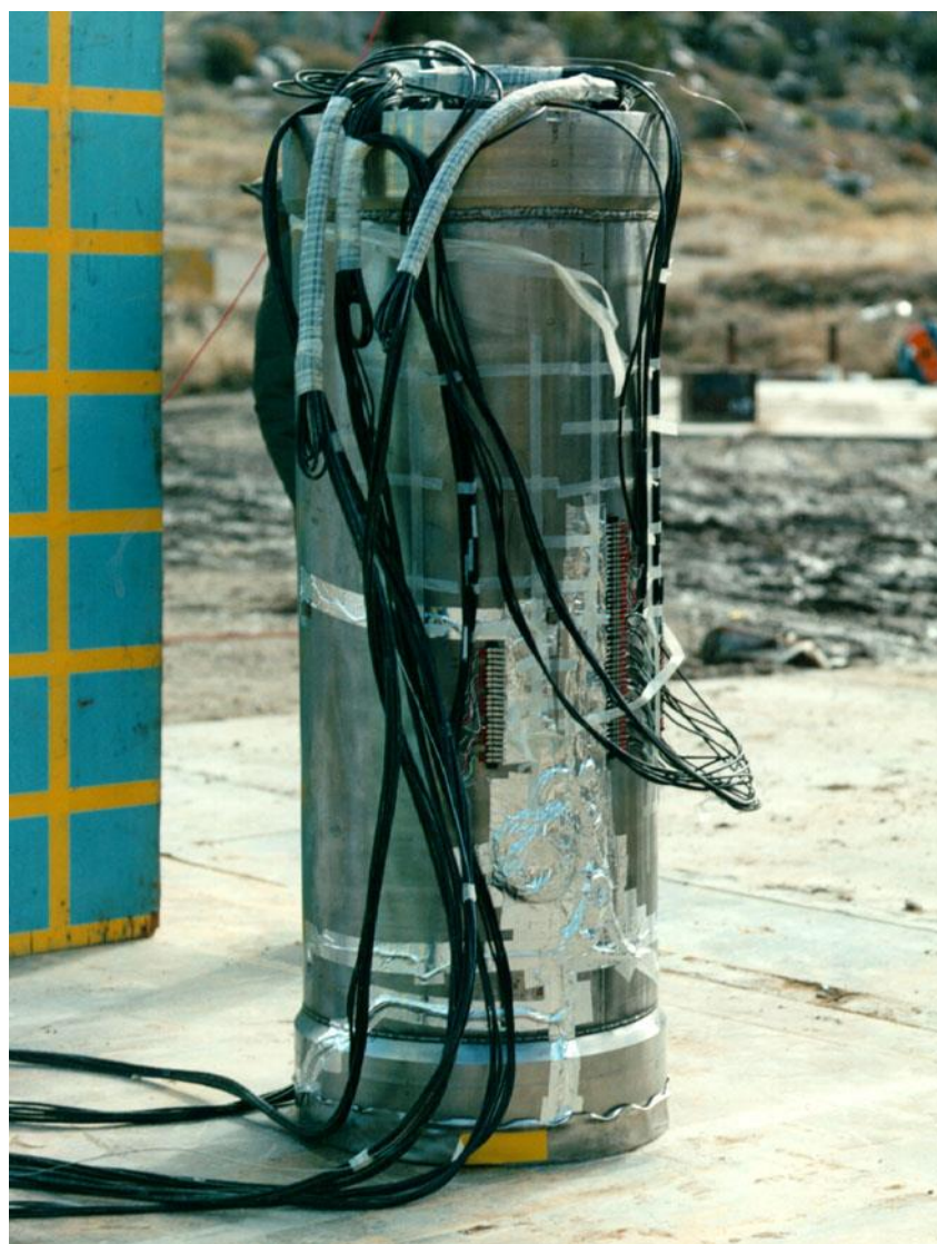
Figure 4 – Deformed shape from the 9-meter drop
