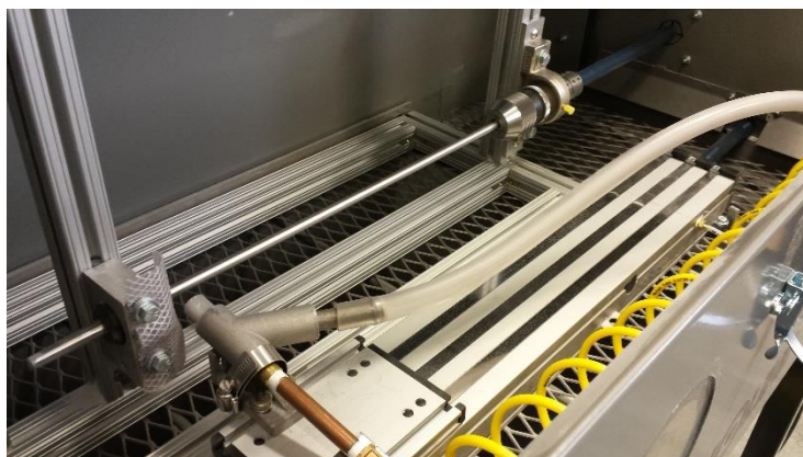
Figure 9: Frit blasting system
