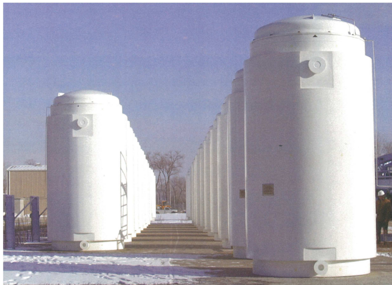
Figure 5 Storage appearance of TN-40 cask
